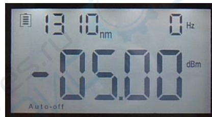
Laser on(output wavelength 1310nm, rated output power-5.00dBm, 0Hz means do not load the frequency
