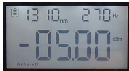
Laser on(output wavelength 1310nm, rated output power-5.00dBm, 270Hz frequency 0Hz means do not load the frequency
